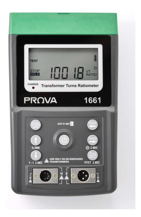
**INTRODUCTION: PROVA 1661** is a precision instrument designed for testing transformer turns ratios across VT, PT, and CT. With wide measurement ranges and fast execution, it is ideal for power system maintenance, manufacturing, and quality control applications. **PROVA 1661** completes all safety checks and displays the turns ratio within 30 seconds, along with excitation voltage, excitation current, and winding resistance of both primary and secondary coils.
